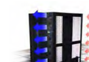
Rack Air Containment
